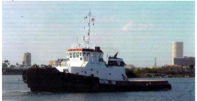
Rev-Lyn Contracting Co. of Boston, MA has sold their 40 passenger crewboat "Harbor Queen" to National Energy Corporation of Trinidad. The vessel was built in 1990 of all aluminum construction by Neuville Boat Works of Louisiana. She measures 46' x 15' x 5.6' and is powered by 2 x GM8V71N main engines producing 600 BHP. The vessel will be repositioned to Trinidad where she will work in the oilfield service sector. Marcon acted as sole broker in the transaction.
